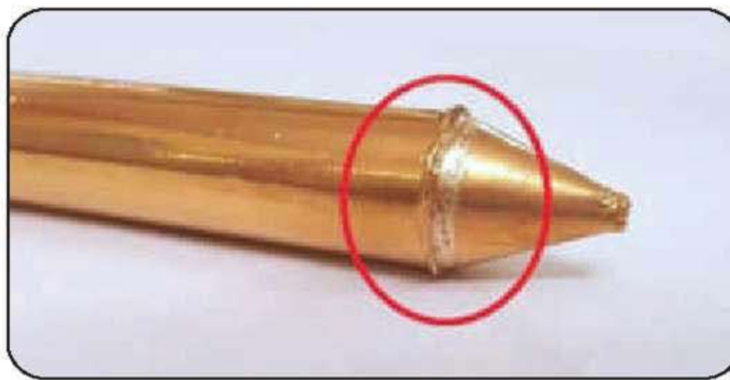
Adhesion Test Clause 9.7.1 (UL 467)
