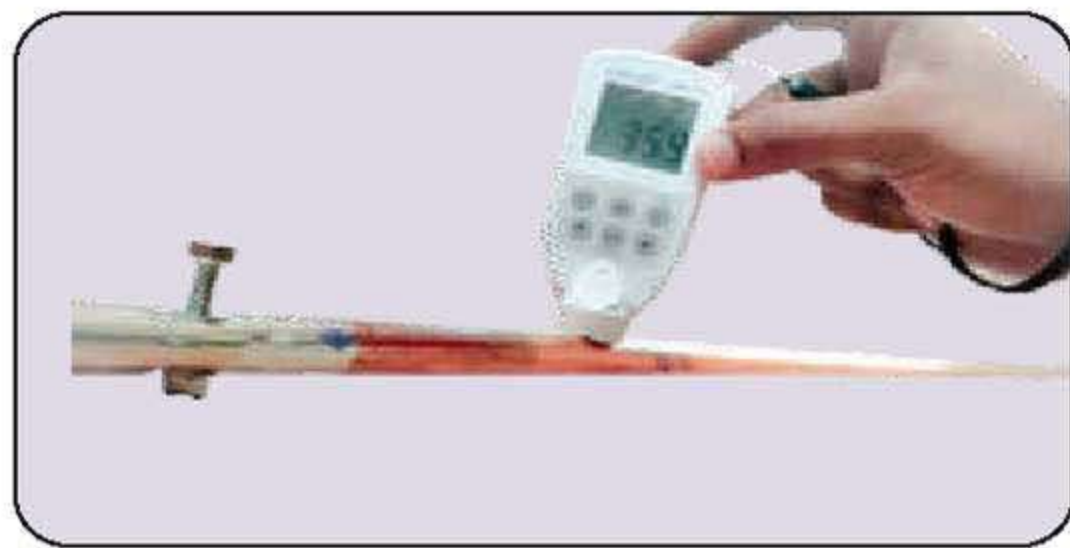
Coating Thickness Test Clause 9.6.1 (UL 467).
